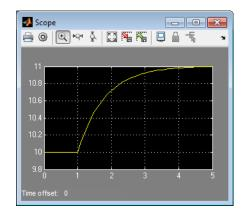
This action updates the Scope window with the response of the nonlinear model with the compensator design. This simulation shows that the rise time is less than 5 seconds and there is minimal overshoot. Thus, this compensator design meets the requirements of less than 5% overshoot and less than 5 second rise time.
