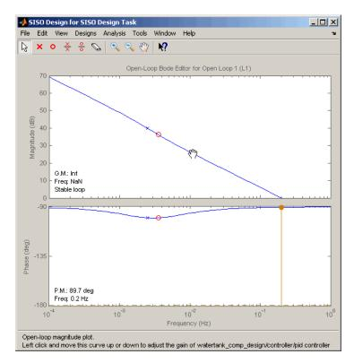
By increasing the gain, you increase the bandwidth and speed up the response. One possible compensator design that meets the tutorial requirements has the following parameters:
