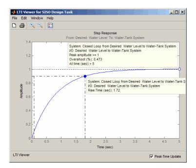
This compensator design satisfies the design requirements of less than 5% overshoot and less than 5 second rise time.
